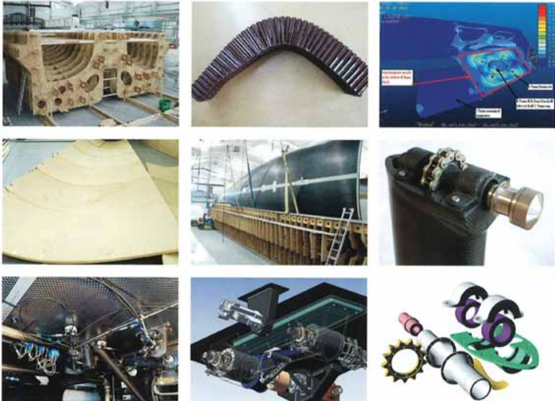
Top row, left to right: the vertically split hull and deck tooling – no plug is needed, the female moulds are all created from scratch; preformed and machined honeycomb sample for the sheer radius; typical component laminate detailing – in this case a bracket. Centre row: preformed foam cores for the slamming areas; with initial hull jointing complete the shell comes out of the half-mould; completed steering head assembly (also lower right), everything is carbon bar the bearing and sprocket. The grinders also provide primary hydraulic power on Ran (lower left/centre) – the complex system required its own team led by Jon Williams and Ian Lovering
