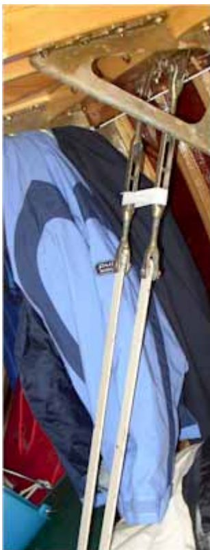
Above: bottom of the diagonal assembly – mast step with turnbuckles connected to the bottom of the connecting plates ( Photo of Bihannic, taken with the permission of Laurent Lafaille )
